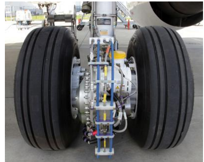
Figure 2: Safran & Honeywell's EGTS
