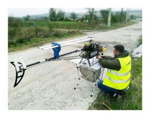
Recently, the company Laserpas used airborne radio controlled drones to complete a survey of the Romanian power grid. The survey overed a total of 358 km of power lines. As a result of the survey effort, the data on locations of power lines was completed, 50 km of reviously undocumented lines were added to records,
